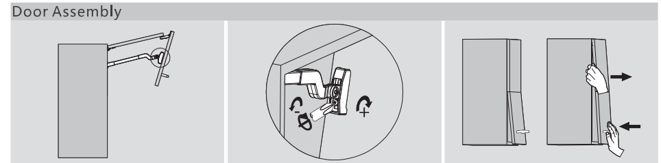
"+" reducing soft-closing time (turn adjustment screw clockwise) "-" increasing soft-closing time (turn adjustment screw counter-clockwise)
